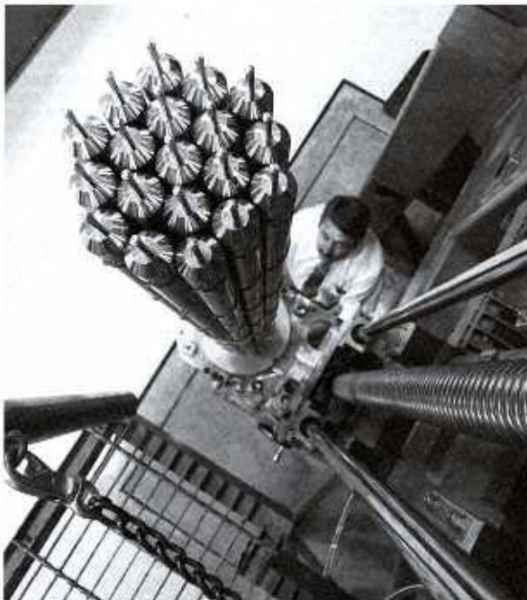
The FFTF test assembly that has produced three beneficial isotopes needed by medical researchers. Craig Knight, of Westinghouse Hanford Company, was the lead fabrication engineer.
