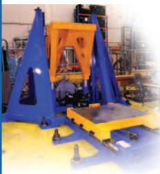
RIM table for seismic testing
