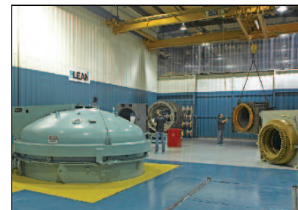
IPS nuclear repair centers in Cleveland and Shreveport have dedicated clean rooms for winding and repairing nuclear motors, applying best practices for Foreign Material Exclusion (FME).
