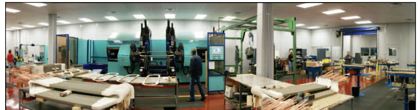
Our VPI and B-stage coils are manufactured in our environmentally-controlled clean room, using our automated taping process and CNC spreader to ensure uniform tape application and precise duplication of coil geometry.
