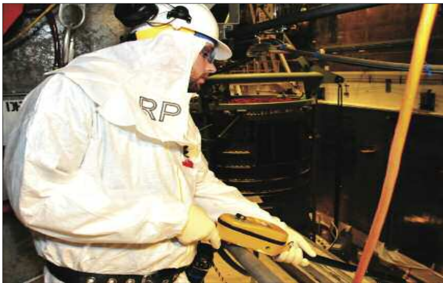
A survey with an extended teletector probe helps keep a radiation protection technician's dose as low as reasonably achievable.
