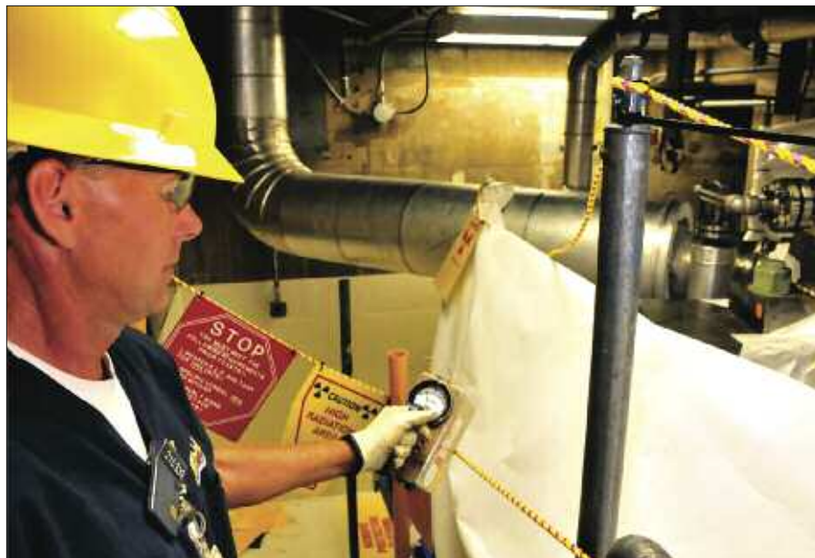
A radiation protection advisor takes a reading to ensure that a high radiation-area boundary meets regulatory requirements.
