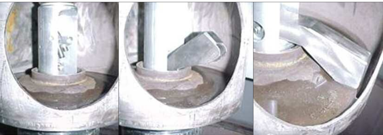
A mock-up of a control rod drive guide tube shows (from left) the Vortex tool partially inserted, the tool inserted with the flush head deploying, and the flush head fully deployed.
