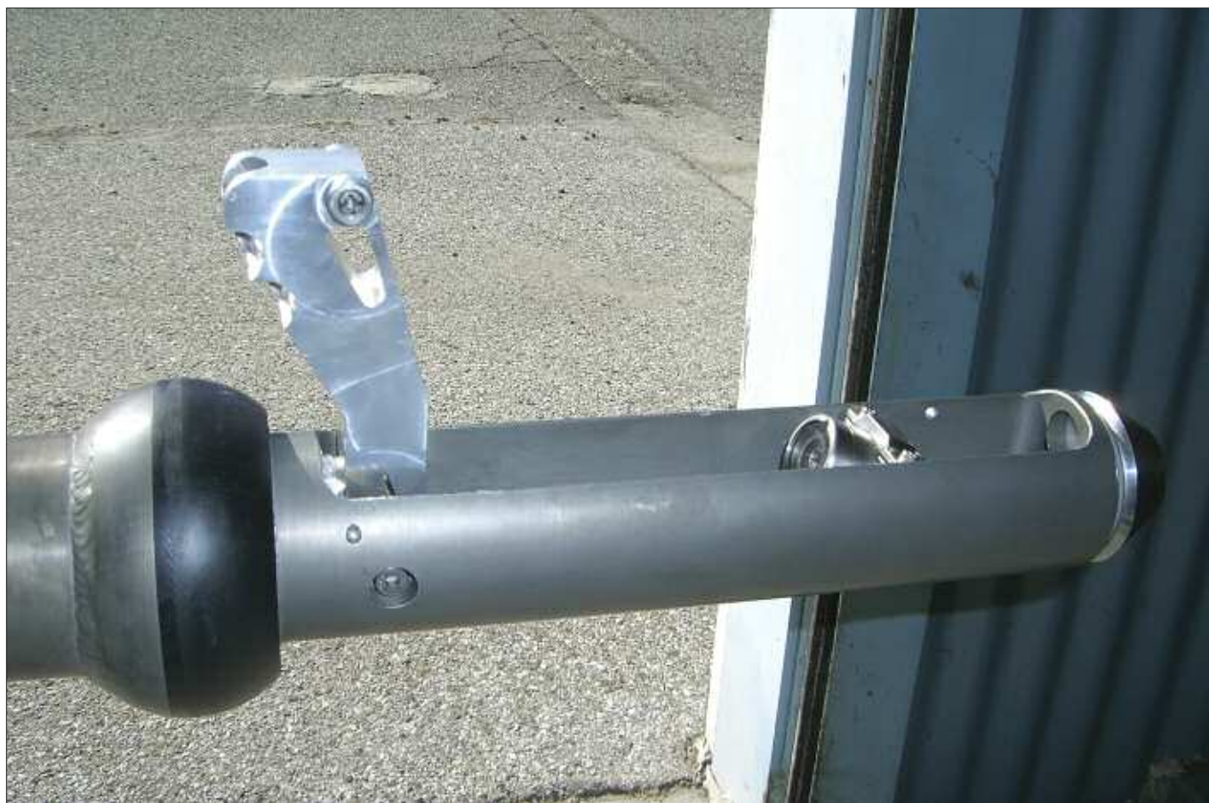
The head of the Vortex tool with the flush head deployed at left and the video camera lens on the right (the tool is usually deployed vertically, but is shown horizontally for display purposes). (Photos: Exelon Generation)
