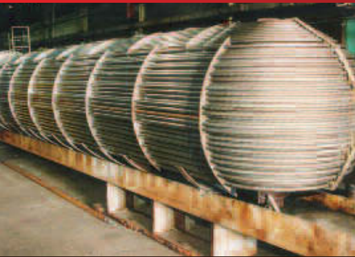
ASME Section III Class 2 RHR Heat Exchanger
