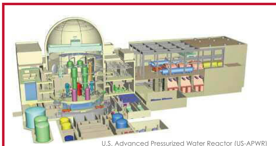
U.S. Advanced Pressurized Water Reactor (US-APWR)
