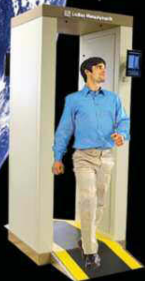
Model 53 Gamma Portal Monitor
