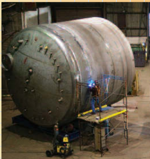
22' Diameter, NQA-1 Stainless Steel Tanks for the Department of Energy
