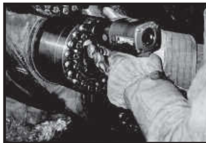
Figure 1: Multi-Jackbolt Tensioners only require hand/air tools to install or remove.
