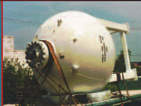
4000 psi, 5 1/2" thick deionized vessel for NASA
