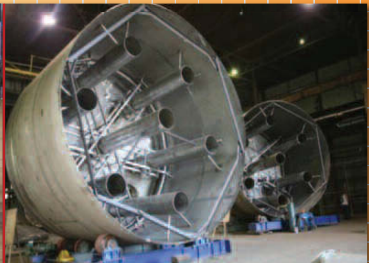
22' Diameter, NQA-1 Stainless Steel Tanks for the Department of Energy
