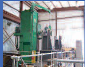
7" Spindle Horizontal Boring Mill with X = 30', Y = 14' and Z = 5'
