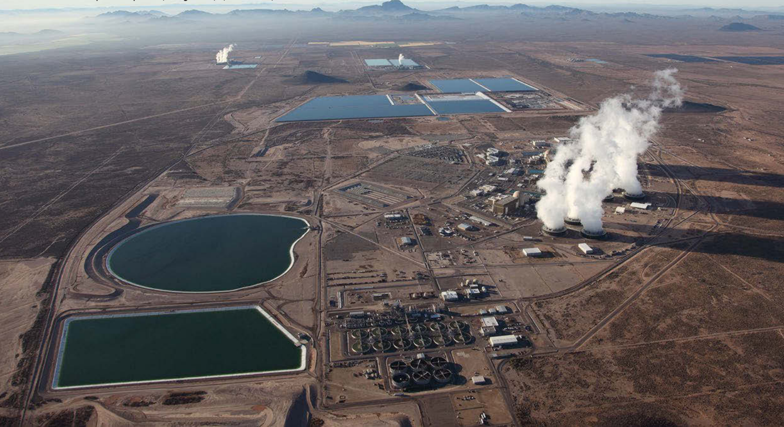
An aerial view of the Palo Verde site, including two reservoirs (foreground) and evaporative ponds (background). (Photo: APS)
