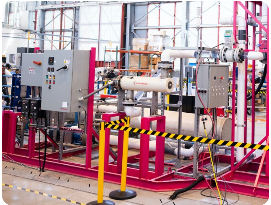
The Engineering Test Unit Demonstration Experiment (ETUDE) test stand validates integral hydrodynamics performance and pebble fuel recirculation methods. Image: Kairos Power
