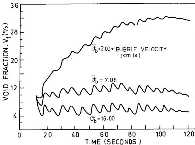
Fig. 4. Computed time variation of void fraction obtained from analysis of experimental data.
