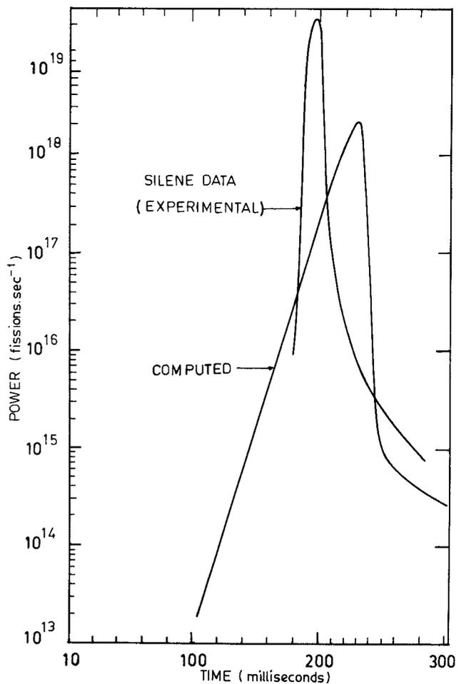
Fig. 1. Power behavior in pulse operation of a homogeneous solution reactor.
