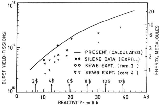
Fig. 2. Variation of total energy in burst as a function of injected reactivity in pulse operation of three homogeneous solution reactors.
