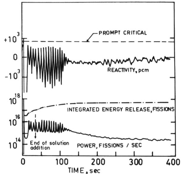
Fig. 3. Time variation of instantaneous power, integrated energy release, and reactivity during a typical free evolution power excursion in a homogeneous solution reactor (experimental).
