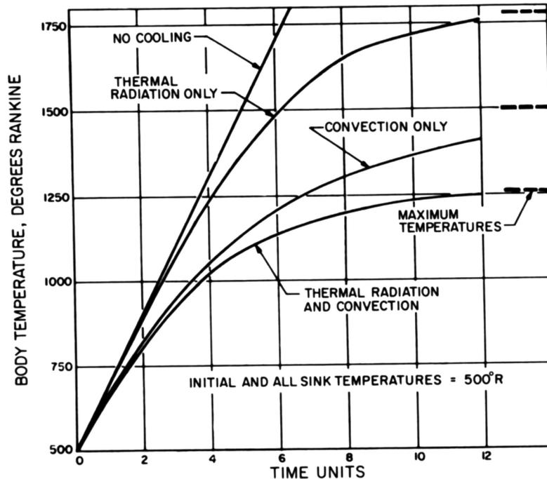
FIG. 2. Thin body heating with various simple-step inputs
