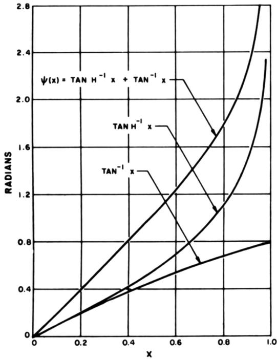
FIG. 1. Functions for thin body cooling by thermal radiation only.
