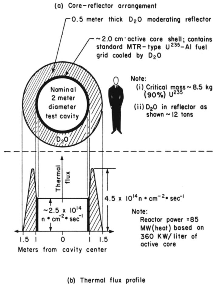
FIG. 1. Core-reflector arrangement and thermal flux profile for a typical cavity test reactor.
