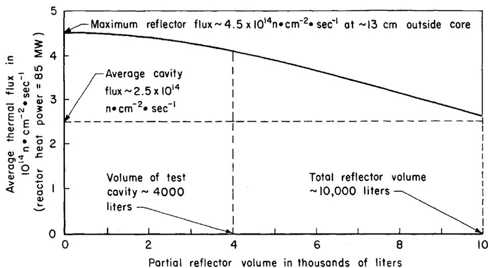
FIG. 2. Average thermal flux in various partial reflector volumes.
