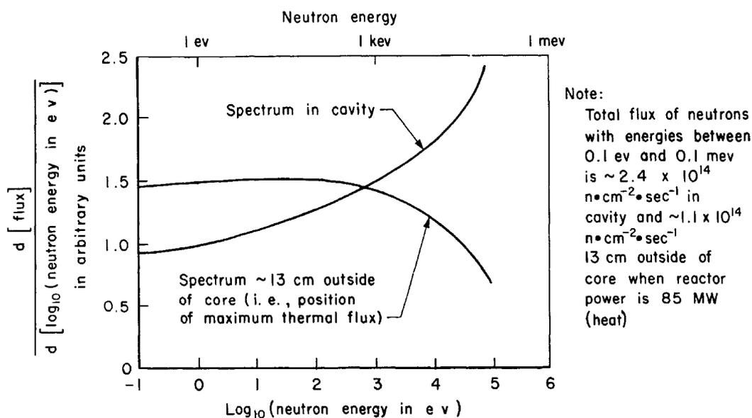
FIG. 3. Spectrum of "slowing-down" flux.
