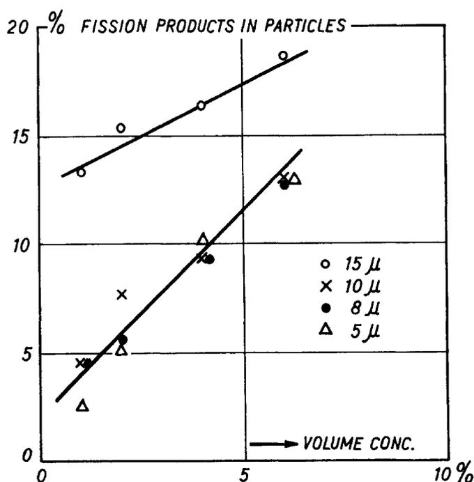
FIG. 1. The percentage of fission products left in the solid as a function of the volume concentration of uranium dioxide suspensions of different particle sizes.
