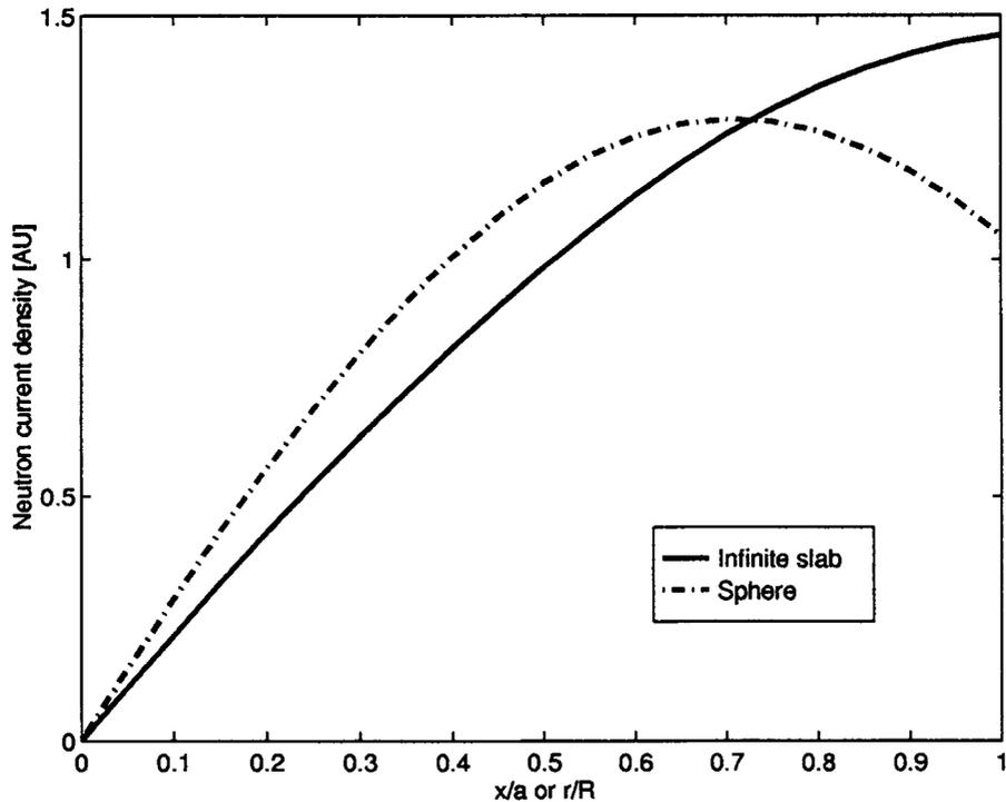
Fig. 4. The neutron current density as calculated from the transport equation for a slab and a sphere with 20 mean-free-path thickness and diameter, respectively.
