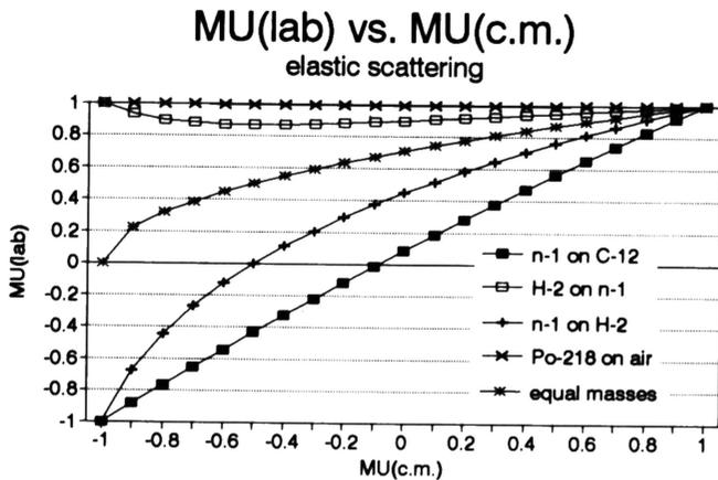
Fig. 1. Relationship of cosines of scattering angles in c.m. and laboratory systems for various mass ratios.
