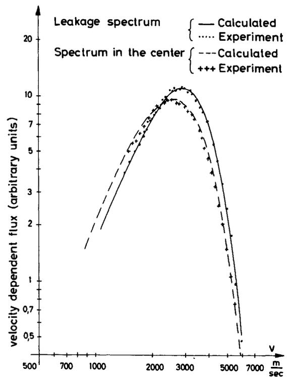
Fig. 2. Calculated velocity-dependent neutron fluxes of a pulsed experiment in a 2.7-cm slab compared with the results of an essentially equivalent experiment.
