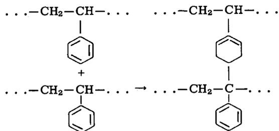
Cross-linking begins to influence polystyrene even when only 0.6 bonds per molecule have been formed. Such samples retain their form and will not melt at 250 C. When three bonds are formed
