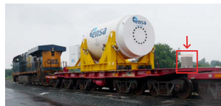
Rail shipment of a transport cask with ARG-US TRAVELER in weather-proof enclosure, 2017.
