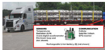
ARG-US TRAVELER remote monitoring system on truck shipment of fuel-assembly containers, 2019.
