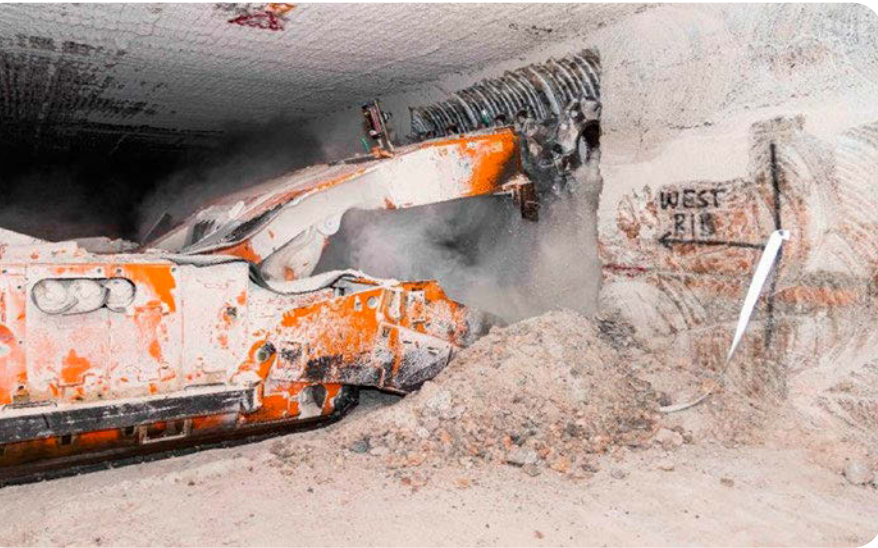
A continuous miner machine cuts into salt rock as mining begins on Panel 11, one of WIPP's next waste disposal panels. (Photo: DOE)
