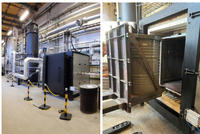
Figure 1. inDRUM Demonstration facility at Studsvik for simulated waste (left) and a drum being loaded into the container treatment unit (right)
