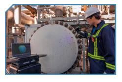
trial, complex geometries, such as elbows, nozzles, pressure vessel heads, tank floors and valves. Creaform's metrology-grade 3D scanners for NDT applications have been proven to measure up to 80 times faster than manual measuring tools. Even better: they can be used by technicians of varying skill levels without any background in metrology or 3D scanning.
