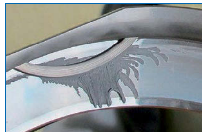
Face seal damage caused by electrostatic erosion.
