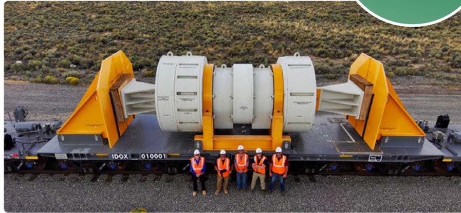
The Atlas railcar carries a test load simulating a shipment of spent nuclear fuel. (Photo: DOE)
