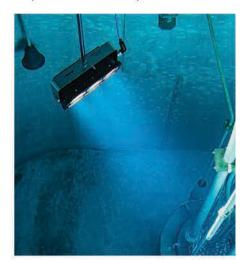
The 85,000 lumen BIRNS Lumena-6<sup>™</sup> is an advanced, intensely bright seismically qualified nuclear underwater LED floodlight that reduces fuel handling costs by bringing daylight illumination to reactor cores, fuel transfer canals and storage pools. It has an integrated power source and is certified for use in water to 70°C without life reduction.
