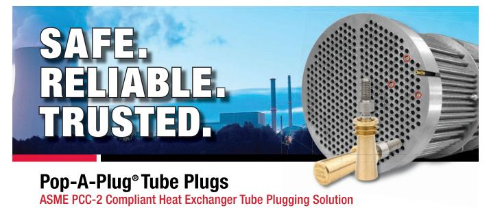
Trusted by Nuclear Power plants around the world as their preferred tube plugging method, Pop-A-Plug Tube Plugs from Curtiss-Wright are engineered for optimal performance throughout the lifecycle of heat exchanger equipment. Controlled hydraulic installation eliminates welding and time-consuming pre-/post-weld heat treatments that can cause damage to tubes, tube sheet ligaments, and joints.
