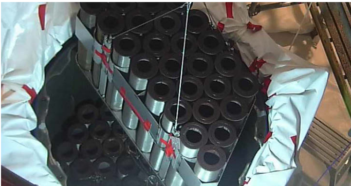
Fig. 3. Top view of a liner loaded with the FLTRSTOR™ system.
